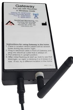
The Gateway is a transceiver (transmitter + receiver) that communicates with the wireless recorder. The Gateway sends the encrypted data via a wireless phone network to the receiving location. Both the recorder and the Gateway are able to transmit and receive data to ensure that encrypted data arrives at its desired location.
